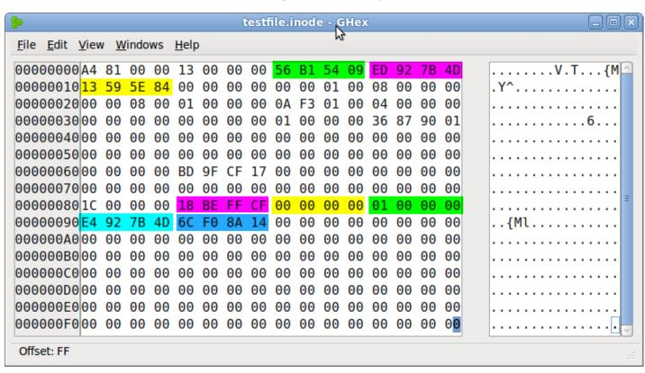
Counting from zero at the start of the inode, here are the byte offsets and meanings for the various highlighted fields:
